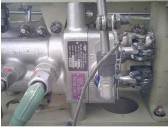
Figure 1: Serviceable BCV with both pushrods contacting input linkage.
