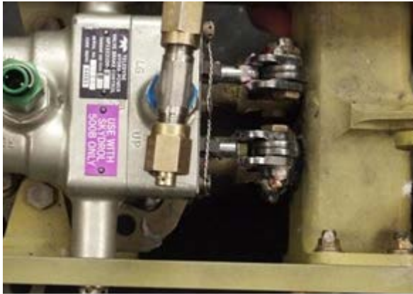
Figure 2: Lower piston with broken spring as lower pushrod not contacting input linkage.
