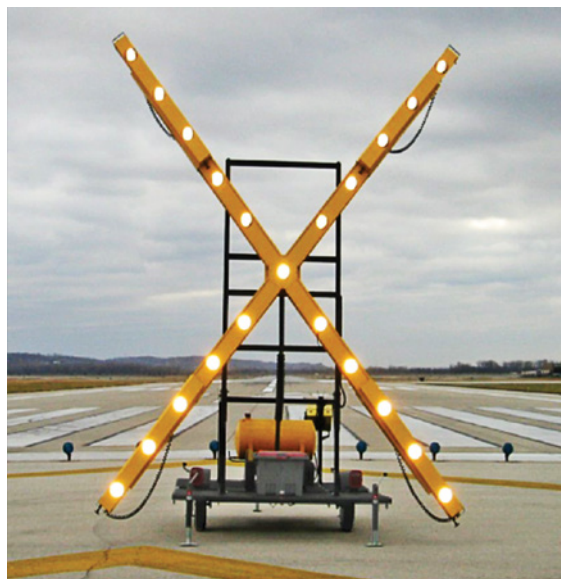
Figure 5.12—Lighted “X” Marking a Temporary Full-Length Runway Closure
