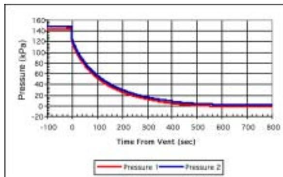
**Figure 4** – Diminishing Propane Pressure in Tank – Test 06-2
