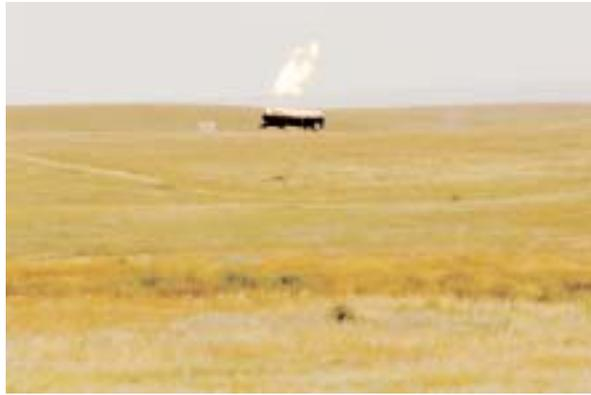
**Figure 1. Initial Vent from Vapour Space**
