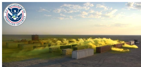
Figure 10. Large scale chlorine release field trial with Utah Valley University Emergency Services, showing the green toxic release cloud and testing environment.
