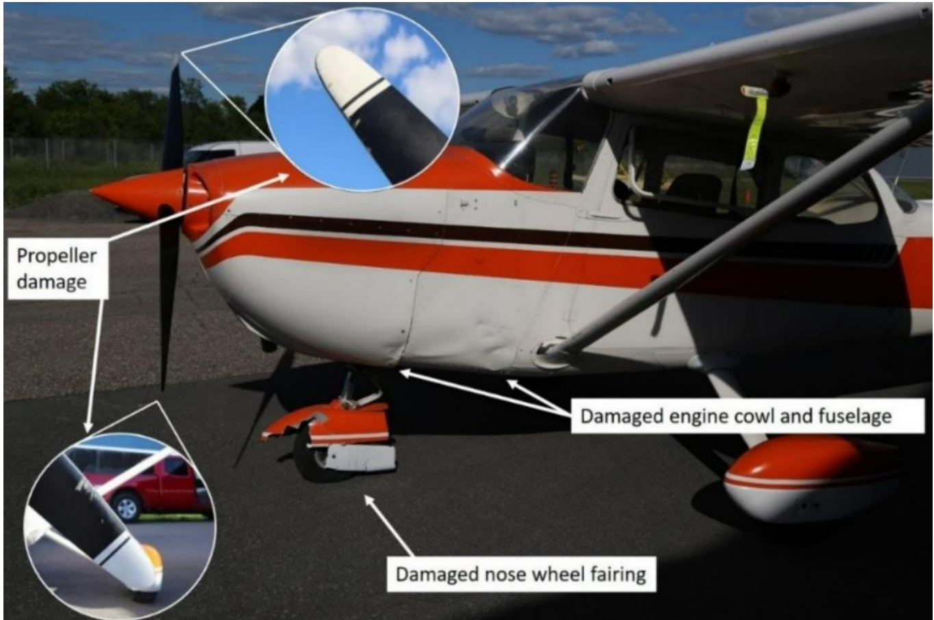
Figure 3. Damage to the Cessna (Source: Ottawa Police Service, with TSB annotations)
