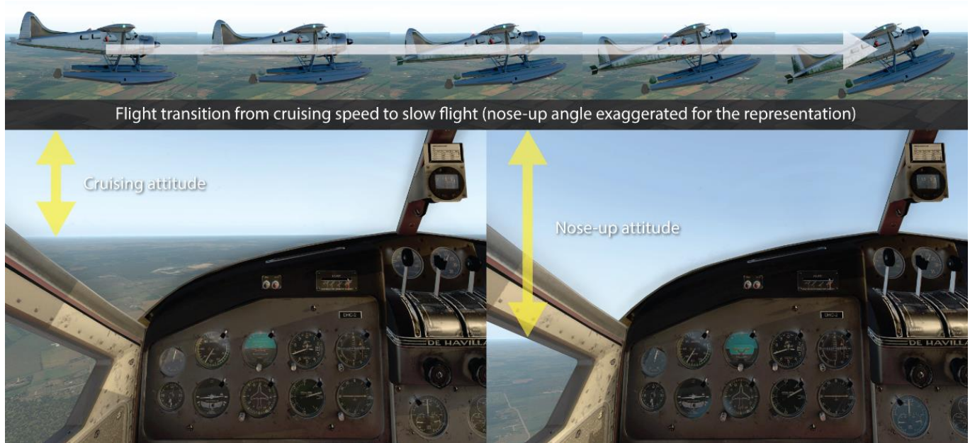
Figure 3. Visual references of the attitude from the cockpit (Source: TSB)
