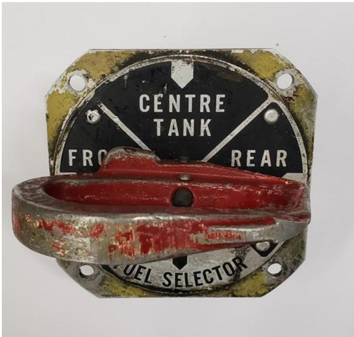
Figure 2. Fuel selector from the occurrence aircraft, with the rear tank selected (Source: TSB)
