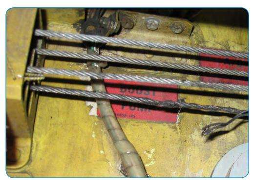
A reminder for personnel that during flight control cable inspection that the entire cable run must be inspected to detect these types of failures. \*
