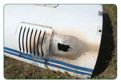
system components are subjected to extreme temperatures and resulting expansion and contraction produce stresses, which often lead to cracks and distortion due to warpage.  $\bigstar$
