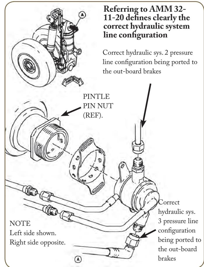
**Referring to AMM 32-11-20 defines clearly the correct hydraulic system line configuration**
