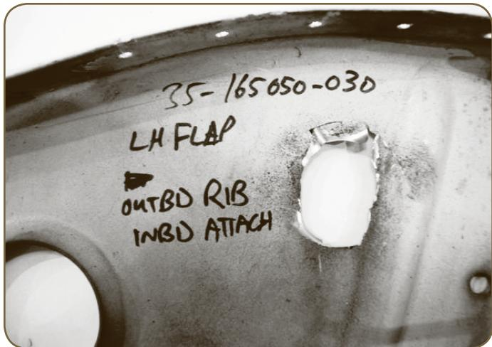
material, 1.27 cm (0.50 inches) thick, eventually failed resulting in a jammed flap.
