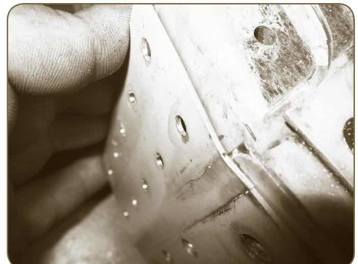
**Elevator Torque Tube - Cracks****SDR submitted:**
