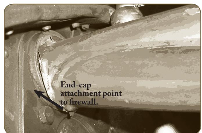
*Failure of this weld could amount to a catastrophic failure of the aircraft.*
