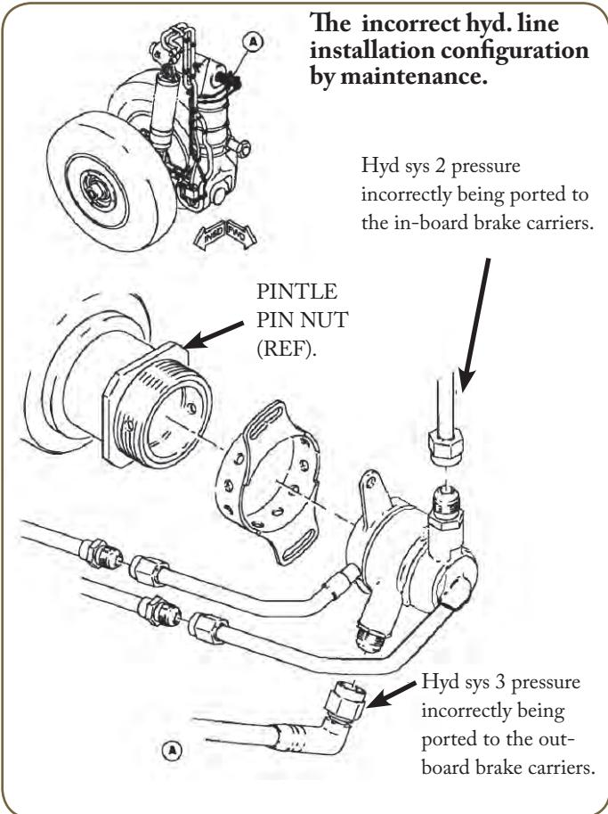
**The incorrect hyd. line installation configuration by maintenance.**
