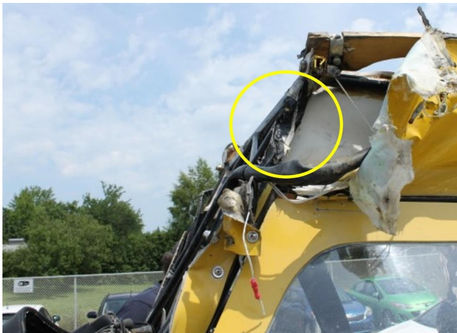
Figure 3: Photo of the damage to the left windshield post caused by collision with the cable (Source: TSB)
