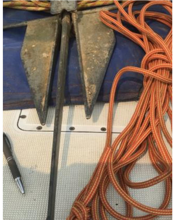
Figure 2: An anchor and rope with a foam-lined blue cloth bag, to be carried in the pilot side float compartment
