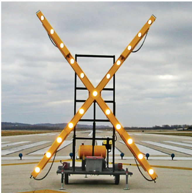
Figure 5.12—Lighted “X” Marking a Temporary Full-Length Runway Closure
