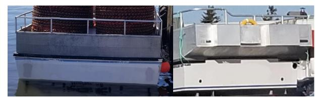
The photos above show examples of removable decks fitted above the vessel's gunwale (washboard).
