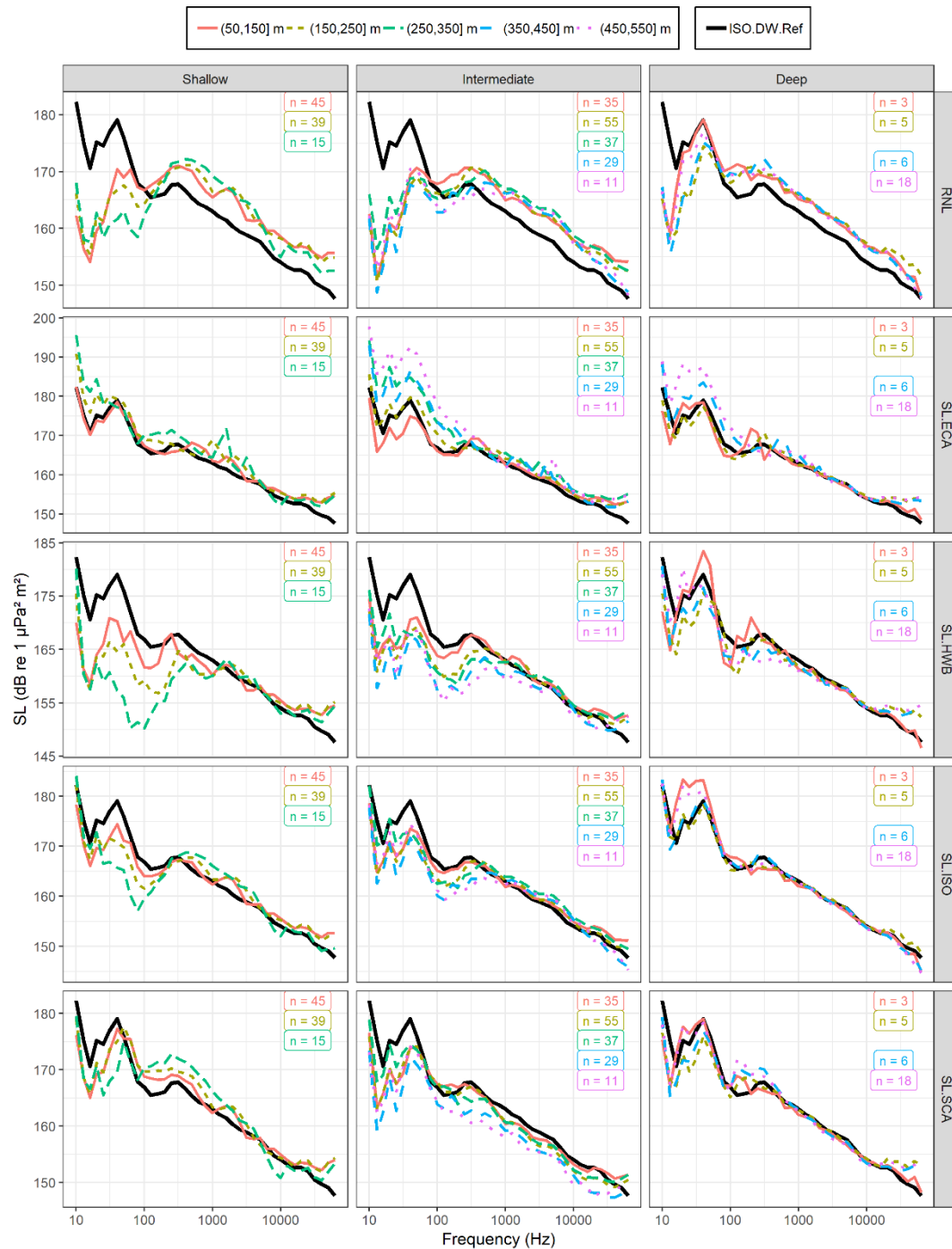
Figure 43. Vessel C: Mean source level versus frequency for single-node hydrophone measurements with speeds through water between 20 and 21 knots. Columns show different sites and rows show different source level (SL) metrics. Coloured lines show different closest point of approach (CPA) distance bins. Black lines show reference measurements (SL.ISO) from the deep VLA. The ‘n’ values indicate the number of individual measurements contributing to the average.
