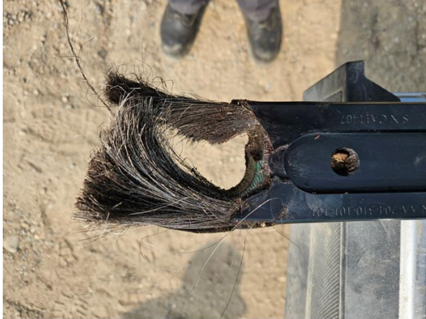
Figure 1 – Failed Airwolf TT strap from the 28 June 2024 accident (Source: TSB 1 )
