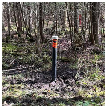
Photo: Well point with protective casing (photo credit CIMA+)
