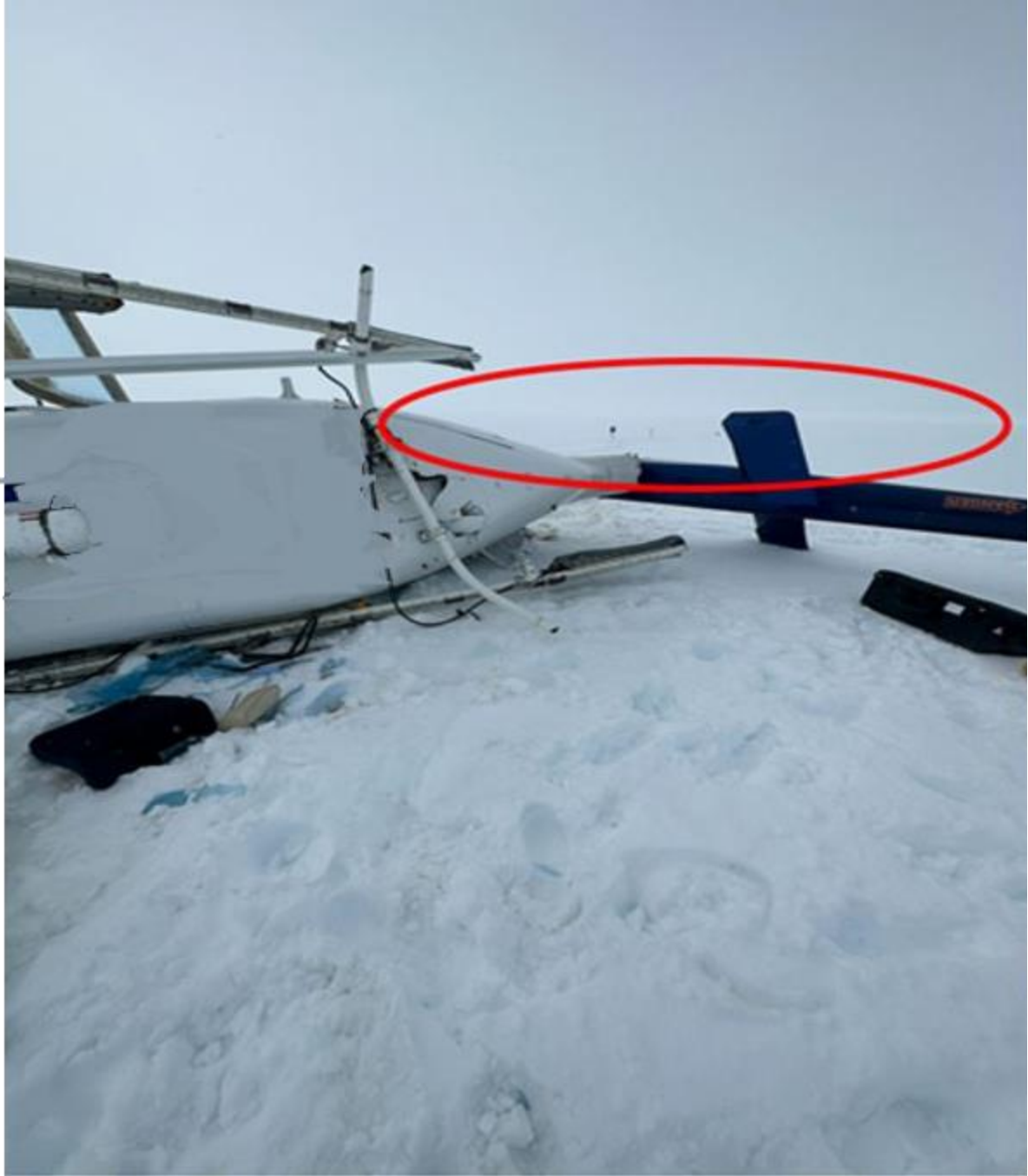
Figure 1: Photo taken shortly after the occurrence, showing flat light conditions with the lack of surface definition (Source: Custom Helicopters Ltd.) Credit: Transportation Safety Board
