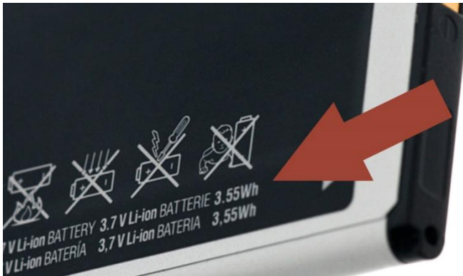
Figure 3: amount of energy (Wh) rating on a battery case
