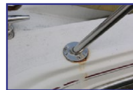
Rust at or on fittings
