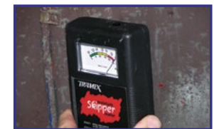
High moisture content
