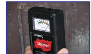
High moisture content
