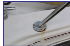
Rust at or on fittings
