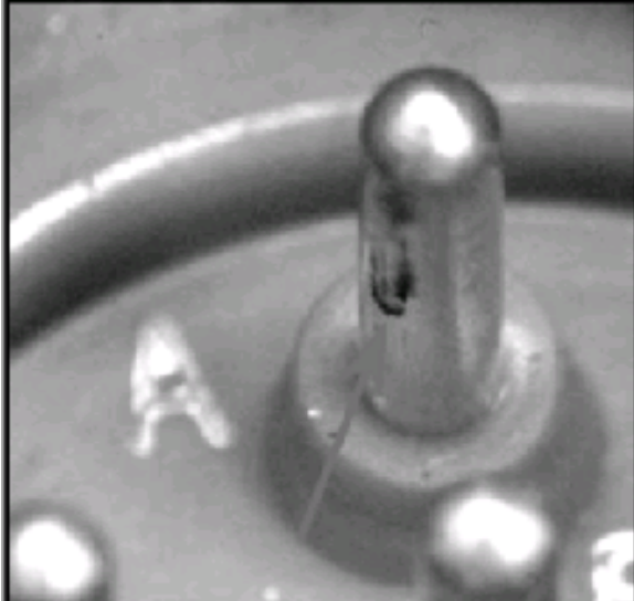
Pin Fretting and Oxidation Usure de contact et oxidation des broches
