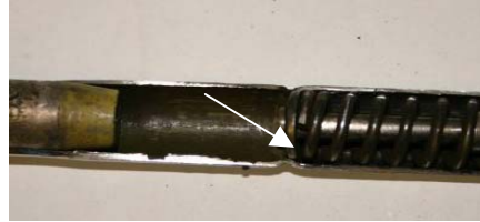
Photo 3: View of washer in normal position/ Photo 3: Vue de la rondelle en position normale
