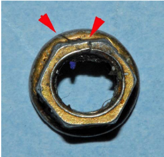
Figure 1; A typical finding of a cracked MS21042-4 nut due to hydrogen embrittlement.
