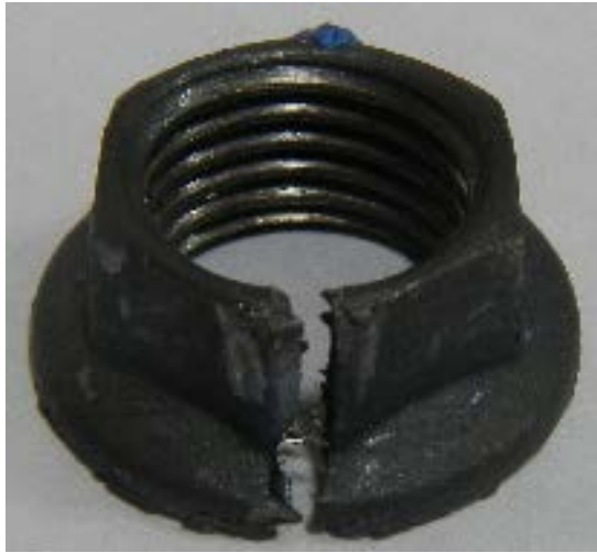
Figure 3; NAS1291-7 cracked nut found by a rotorcraft operator.
