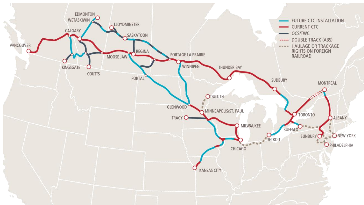
FIGURE 15: CP CENTRALIZED TRAIN CONTROL (CTC) PROJECTS
