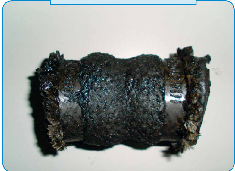
Swollen coupling causing oil loss
