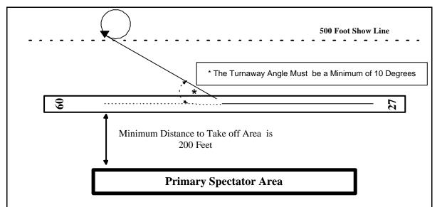
Note: In the above diagram, the runway/take-off area for the CAT III aircraft is less than 500 feet from the primary spectator area. Thus, as per par. 623.07(4)(b) aerobatic manoeuvres are allowed after take-off when a "turn away" is carried out as illustrated above and once the aircraft has reached the 500 foot show line.
