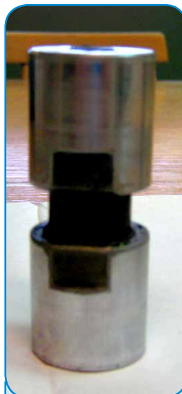
Missing retention nut and bolt threaded end
