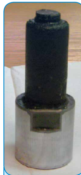
Missing bolt threaded end and extensive corrosion
