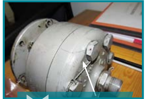
Hydraulic Pump Case Crack Causing Hydraulic Fluid Loss
