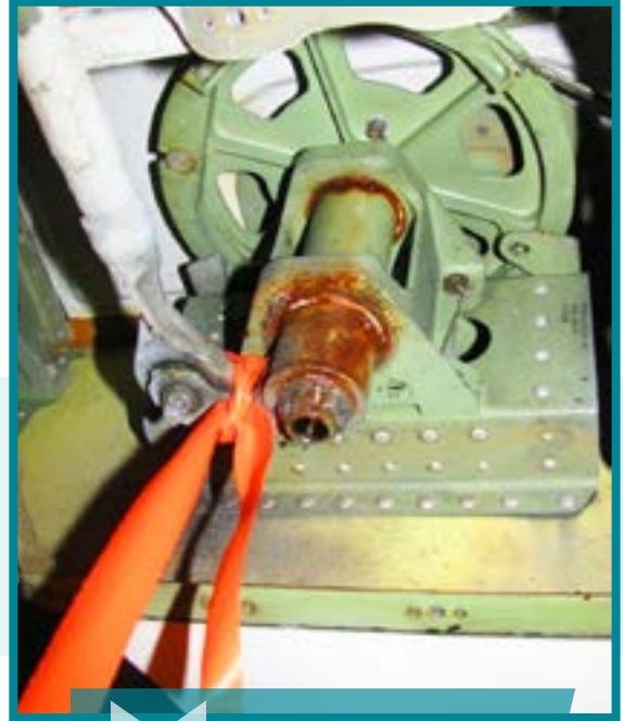
Aileron Quadrant Bearings Severely Corroded
