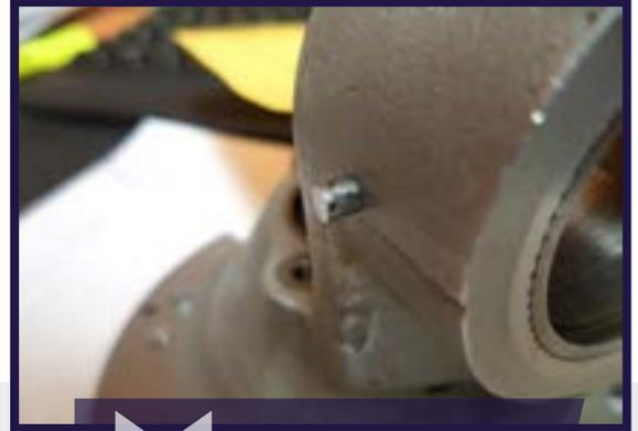
Retaining pin found not staked and backing out of assembly.
