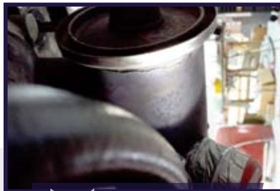
Muffler With a Significant Crack Near the Flange
