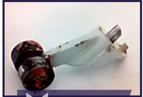
Tail Rotor Counterweight bolt failure
