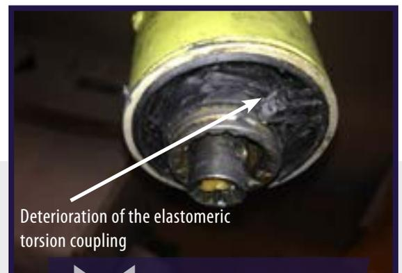
Deterioration of the elastomeric torsion coupling
