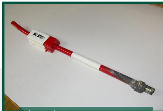
Tuning weight location on the failed tail skid
