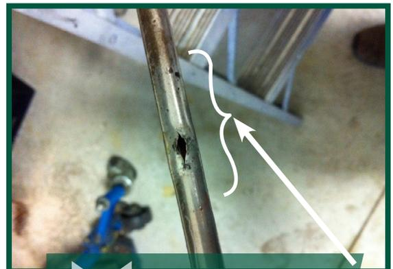
Hydraulic rigid line failure with evidence of the rubber line support block contact area
