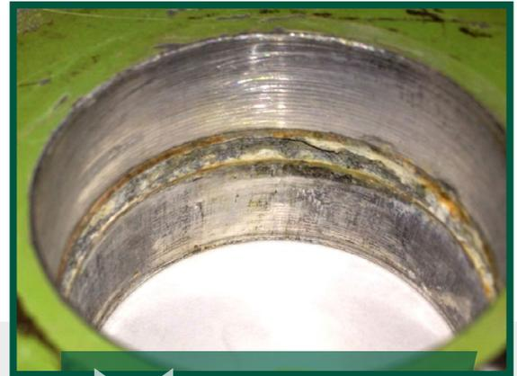
Fitting with corrosion under bushing location
