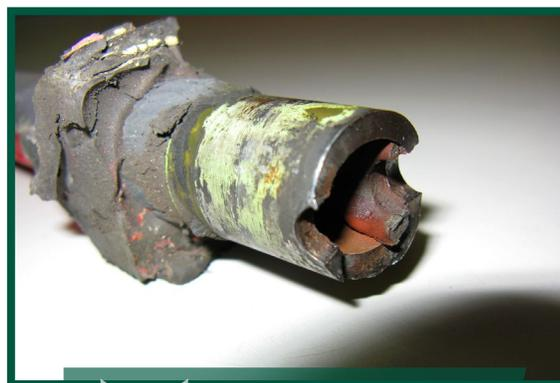
Corroded tail skid assembly failure
