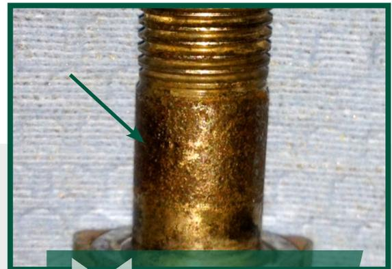
Heavy corrosion pitting of the brake retention bolts
