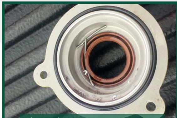
Main transmission oil filter metal debris
