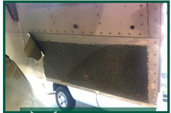
Trailing edge flap panel disbond skin damage and exposed honeycomb
