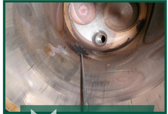
Cylinder bore with indication of coating delamination, while this might not look bad; due to the small clearances this material can cause significant damage
