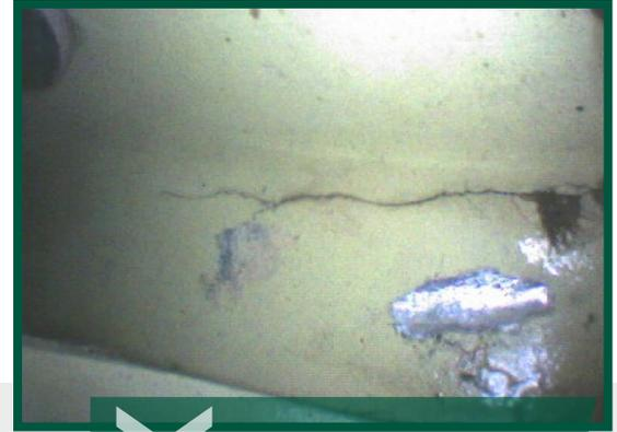
Forward pressure bulkhead cracks found
