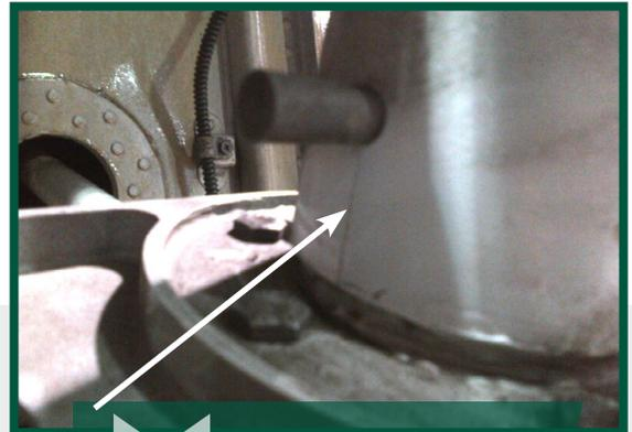
Crack at the taper pin attachment hole
