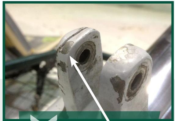
Main landing gear uplock roller lug crack
