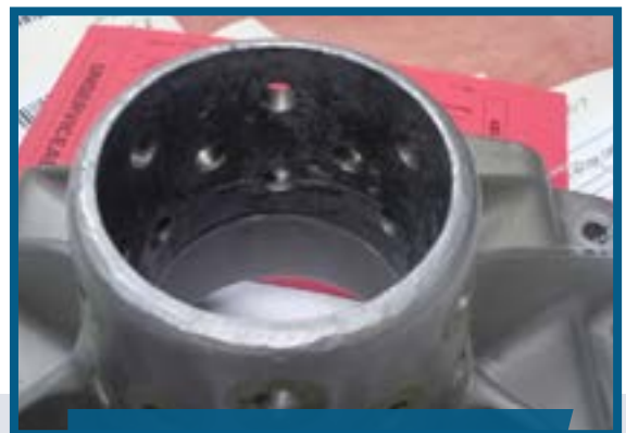
Cracked rudder torque tube coupling
