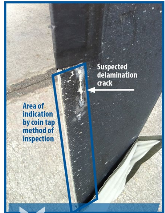
Propeller blade with area of suspected delamination highlighted.
