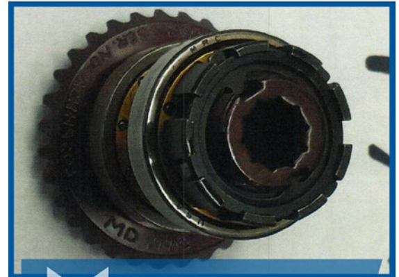
Bearing with improper markings for application.
