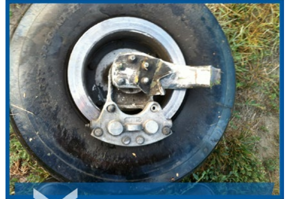
Separated wheel assembly with part of the broken main gear spring still attached.
