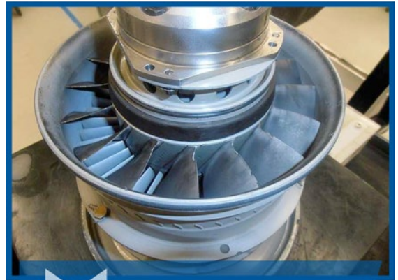
Engine compressor showing foreign object damage to the first stage blades.
