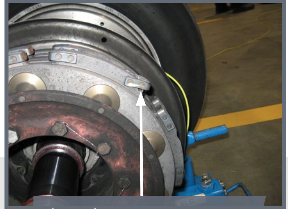
Failed Brake Carrier Rotor Clip
