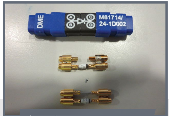
View of both the serviceable and shorted diodes
