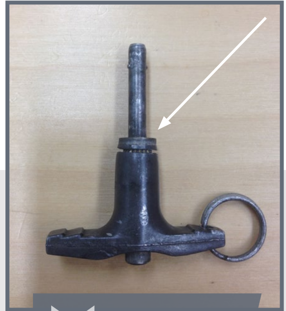
Cracked Release T Handle P/N 204-072-727-013
