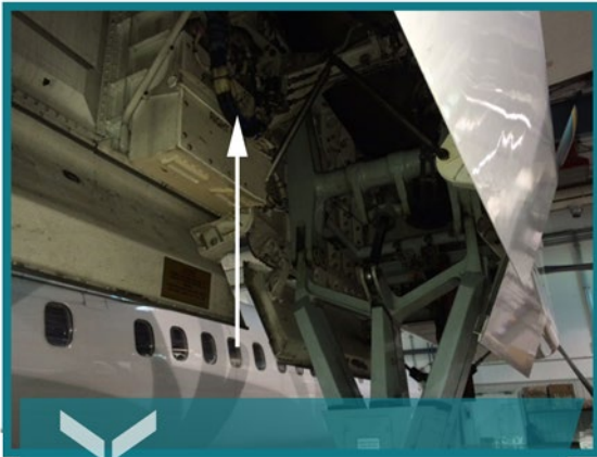
Damaged connector in the right hand wheel well.
