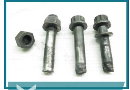
Damaged wheel tie bolts.
