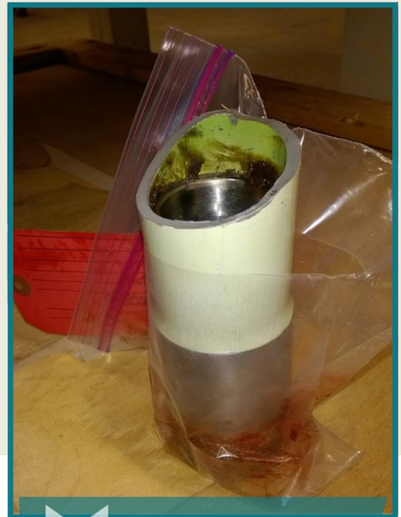
Failed nose landing gear axle piece that broke off.
