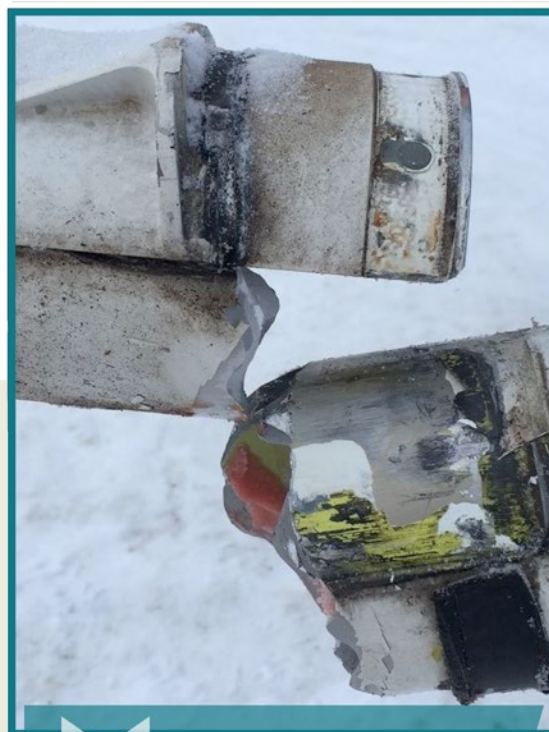
Aft cross tube that fractured under the left hand saddle.
