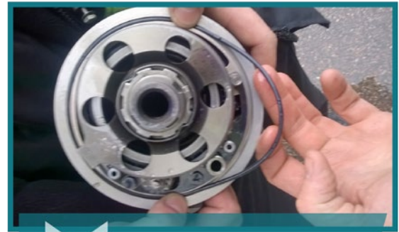
PCU with damaged o-ring.
