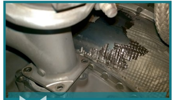
P2.5 valve and High pressure compressor case missing attaching hardware.
