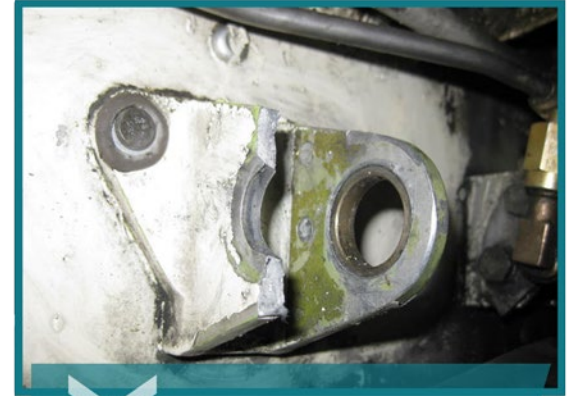
Broken Slat attachment fitting.
