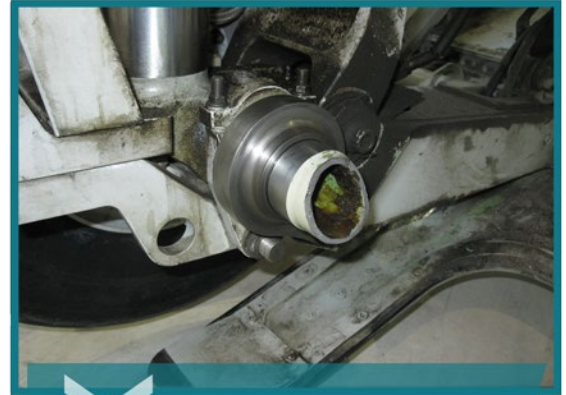
Nose landing gear showing broken axle as seen when the gravel kit is removed.
