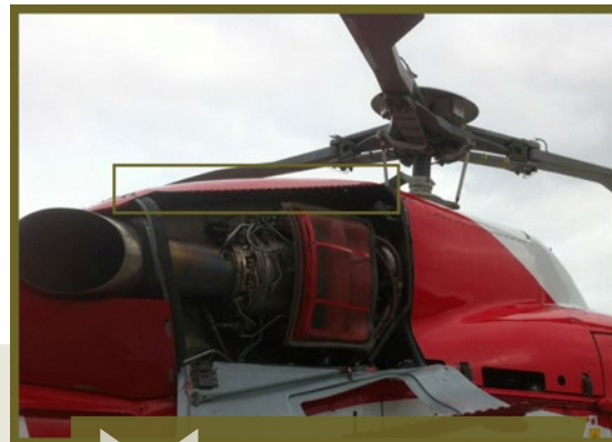
Engine Cowling latched with missing upper hinge pin
