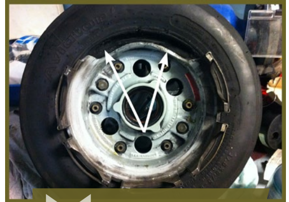
Wheel rim half section missing
