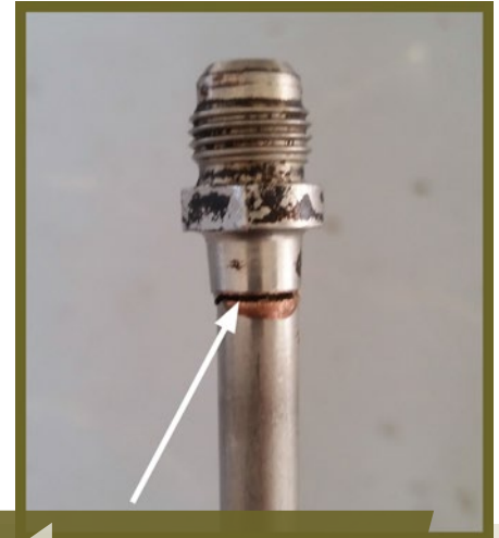
Oil scavenge tube assembly rupture at the flare solder joint
