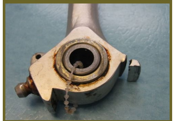
Service door failed hook with broken tab
