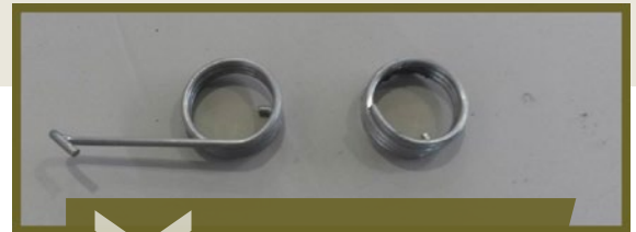
New spring & broken spring
