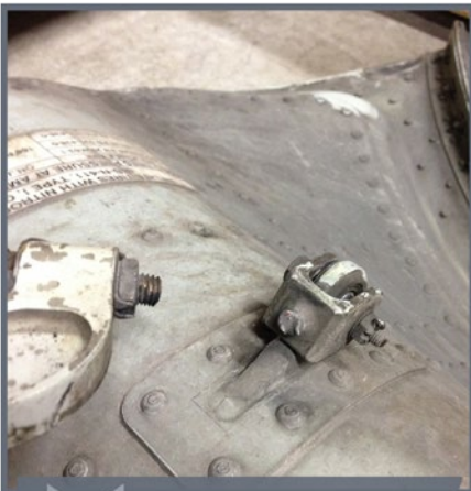
Broken rod end of the main landing gear door.
