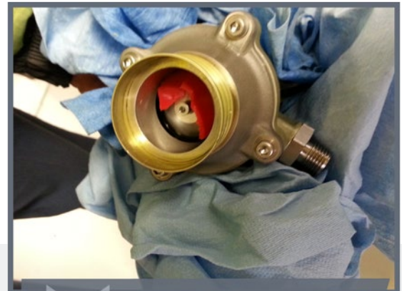
Visible foreign object damage (FOD) in the fuel transfer valve.
