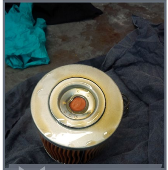
New filter assembly as removed from the factory housing with evidence of damage on the relief spring contact end.
