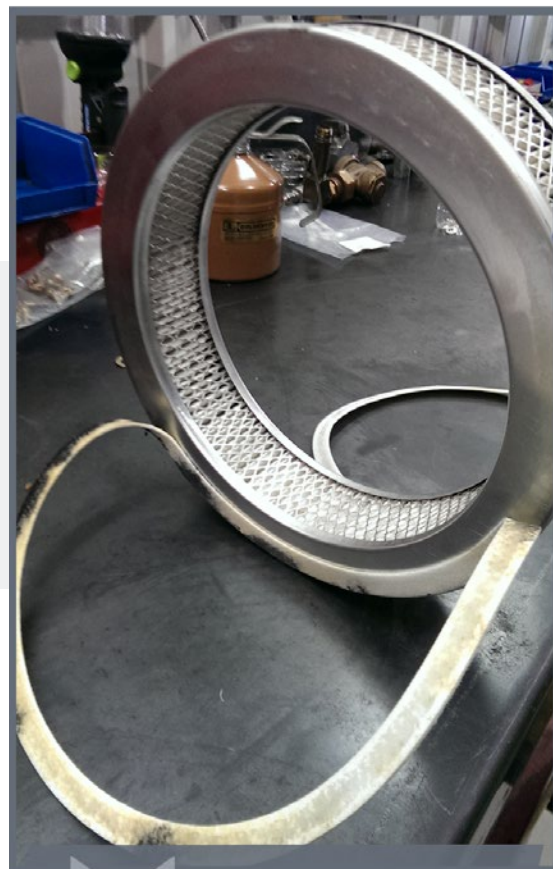
Example of the gasket becoming detached from the air filter.
