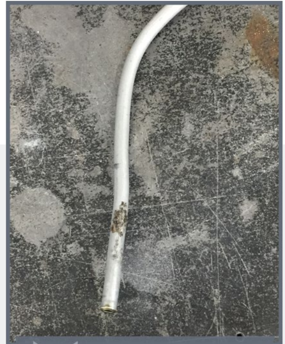
Corroded part number 0700099-37 oil pressure line.
