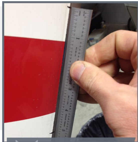
Debonded abrasion strip on tail rotor blade.
