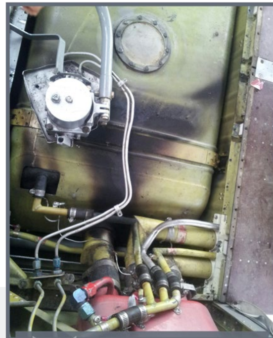
The fuel tank from a DeHavilland DHC-2 MK1 with burn marks on the exterior.
