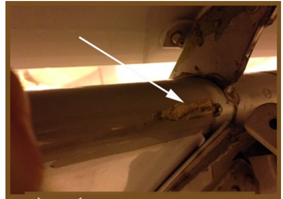
Flap vane leading edge damage incurred by the missing bute-door roller
