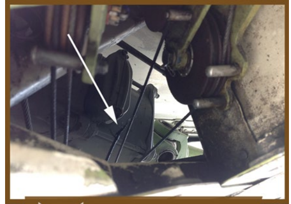
A spoiler control cable that failed after it was in a frayed condition
