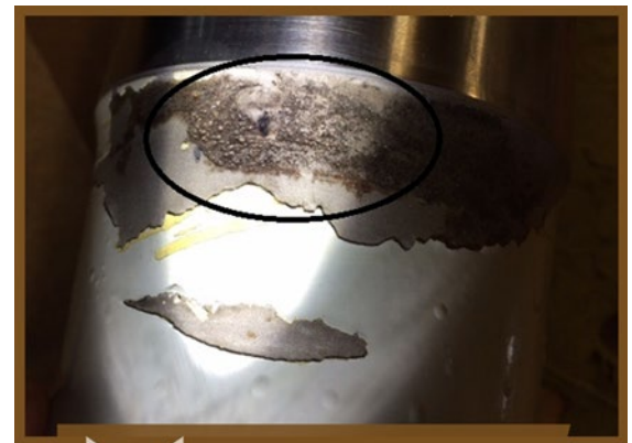
Pitting on surface, measured with optical micrometer, the deepest was 0.022 of an inch (0.5588 mm)
