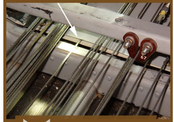
Misrouted engine fuel lever control cable fretting on the aeroplanes structure
