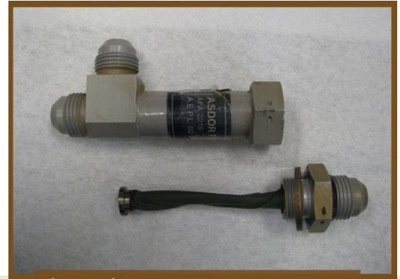
Fuel Scavenge Ejector Filter screen collapsed due to contamination
