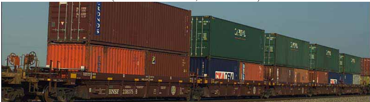
Figure 8 Photo of a 5 Unit Articulated Intermodal Rail Car (Carries 10 Containers, Double-Stacked)
