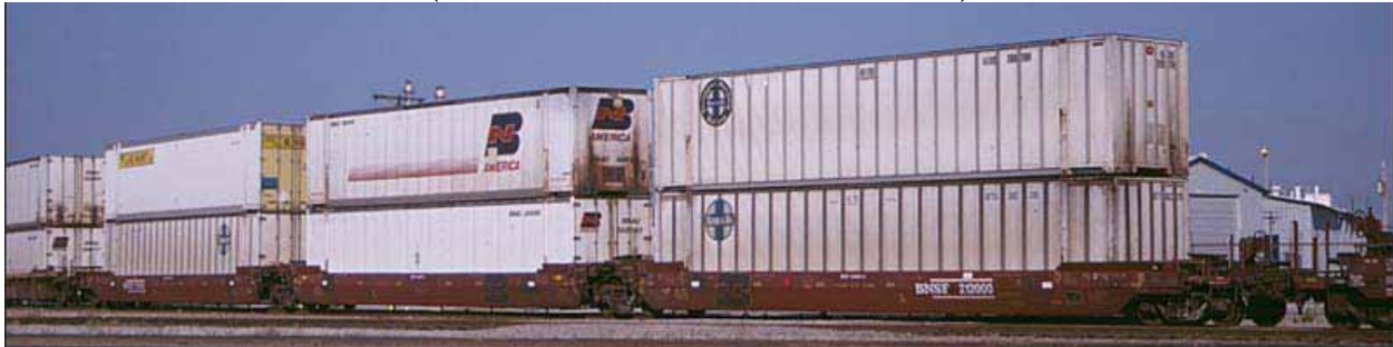
Figure 7 Photo of a 3 Unit Articulated Intermodal Rail Car (Carries 6 Containers, Double-Stacked)
