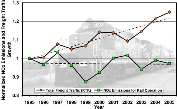
"RTK" stands for revenue tonne-kilometers, which refers to the product of the weight (in tonnes) of revenue commodities handled and the distance (in kilometers) transported.
