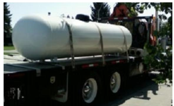
*Stationary tank loaded onto a vehicle*
