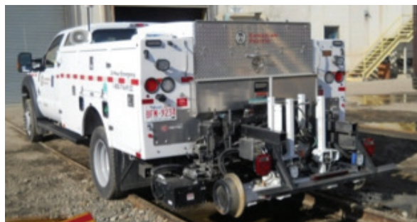
Hi-rail Track Geometry truck
