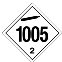
Placard for UN1005, ANHYDROUS AMMONIA SOR/2014-159
