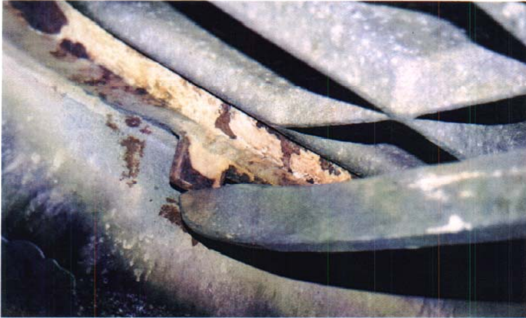
Photograph 3 – The cross bar was tightened by the operator from his position on deck and outside the compartment. He was completely unaware that it had come to rest on top of the wedge piece.
