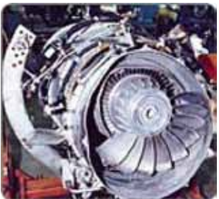
Destroyed jet engine due to bird strike. Aircraft on takeoff phase, 50 ft. AGL, 140 knots.
