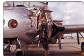
Bird strike damage due to Turkey Vulture
