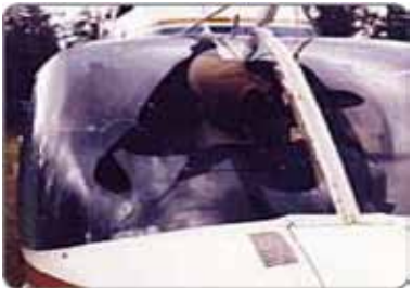
Jet Ranger bubble destroyed by bird strike.
