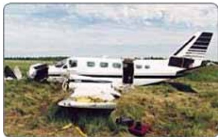
Fort Frances, Ontario (1994) Crash on takeoff resulting from engine damage caused by gulls.
