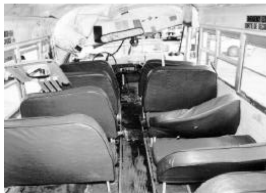
Deformation to seat backs
