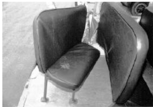
Forward deformation of bus seats
