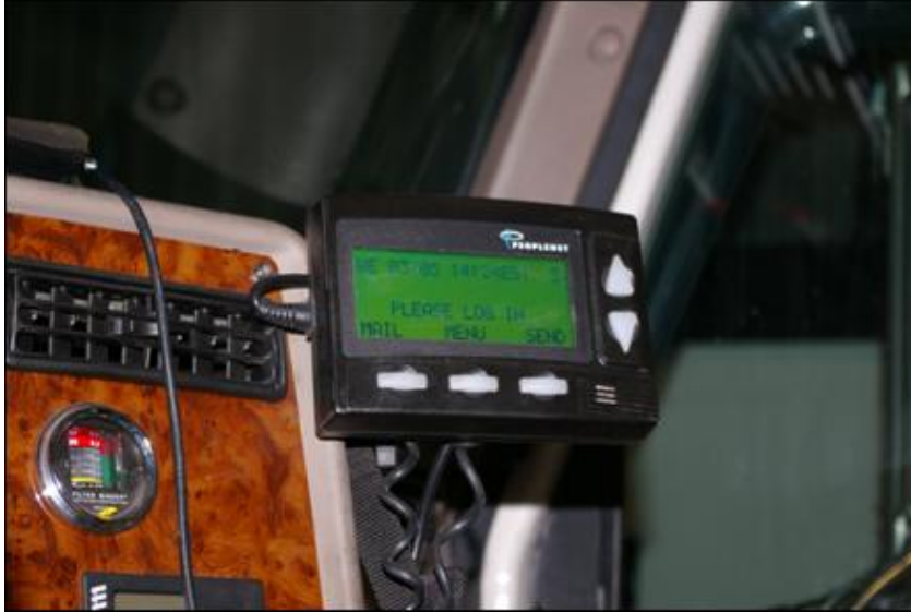
Figure 2 – PeopleNet interface used in the private carrier's trucks
