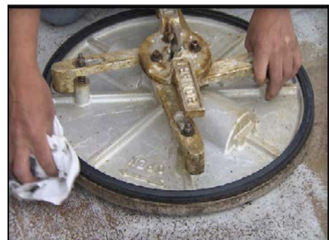
Figure 1.0. Seals around man-hole covers are amongst the many items associated with closing appliances that must be checked regularly and properly maintained. (Courtesy of the Canadian Council of Professional Fish Harvesters (CCPFH)).
