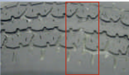
A tire must be replaced when the tread wears even with the tread wear indicator.
